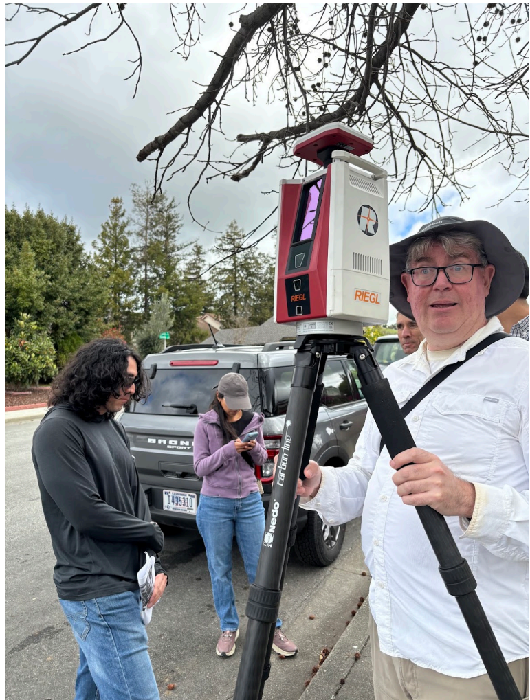
Capacity building in action -- Steve DeLong showed the March 2026 workshop how to find the Alignment Array markers (NOT TRIVIAL!). Jessie Vermeer USGS demonstrates high precision measurement to Travis Orloff. Gareth Funning (UCR) enthusiastically operates the laser scanner to collect point clouds on displaced curves. Rezagene Milani (USGS/SJSU) with the GPS Antennae Dylan Cardiff debates the set up with Belle Philibosian.
