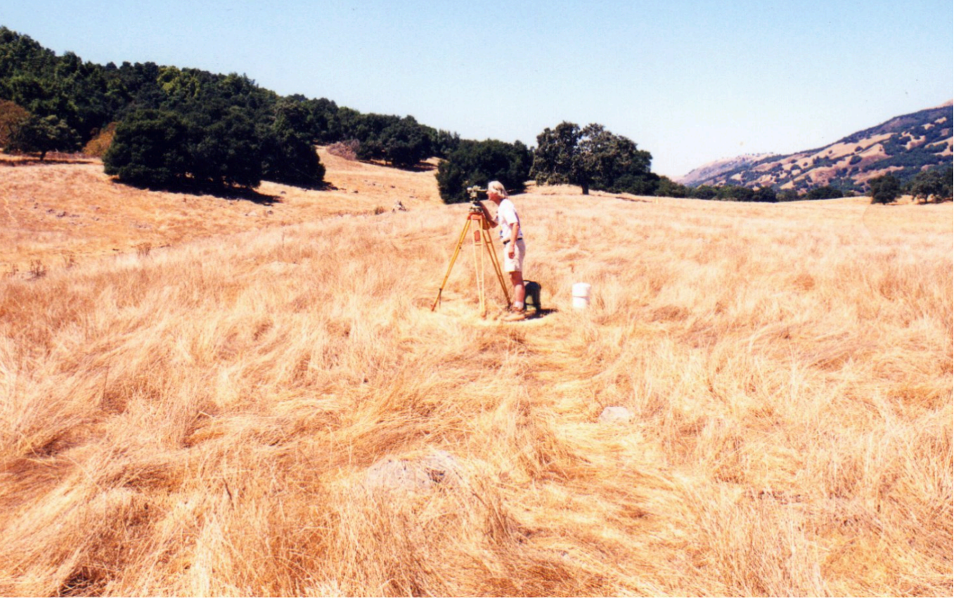
SFSU Personnel measuring alignment array at Mendoza Ranch, across the axial trough of the central Calaveras Fault. Photo presented by Forest McFarland.
