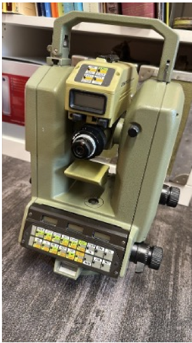
left: AA stats. (S. DeLong) right: Wild T2000 theodolite: Angular resolution 0.5" or ~0.24 mm at 100 m.
