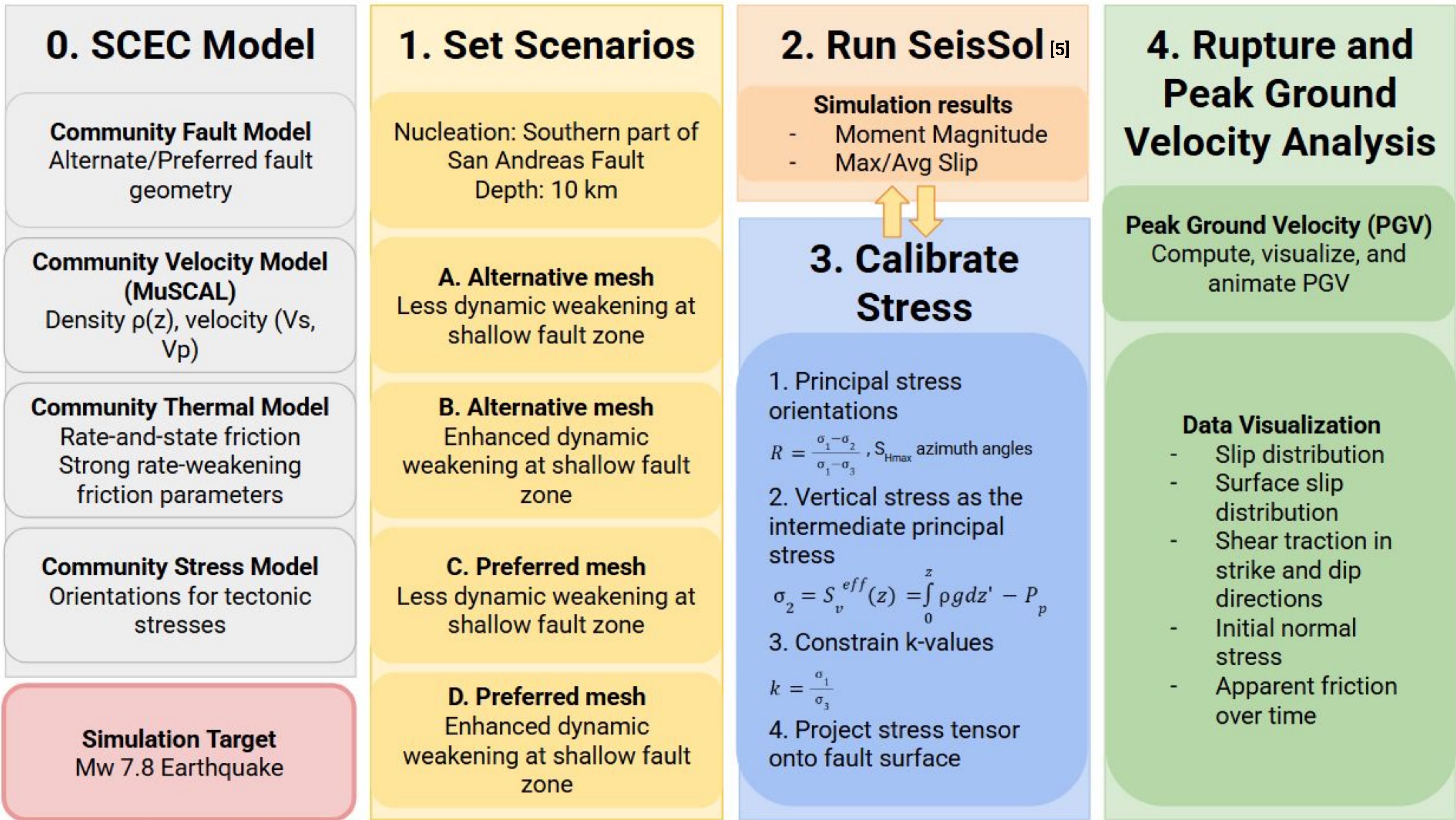
Figure 5: Workflow for developing M7.8 simulations and ground-motion maps
