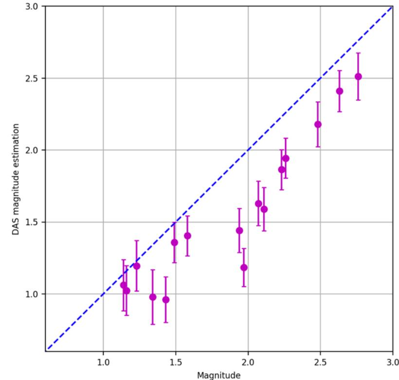
$$M_L = \log_{10}(S_{DAS} \times 10^6 \times GL) + 2.56 \times \log_{10} R - 1.67$$
